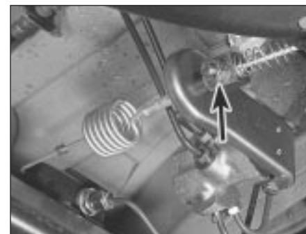
22.3 Light-laden valve linkage adjustment locknut (arrowed)
