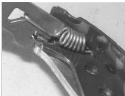
6.7b Detach the adjuster strut
