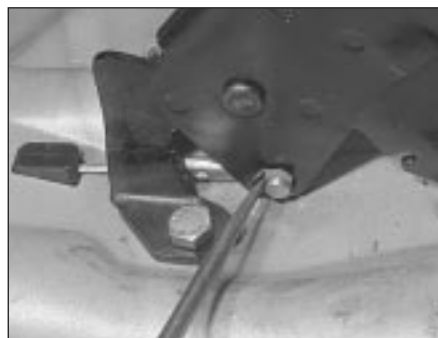
17.9 Removing the handbrake primary cable clevis pin securing clip
