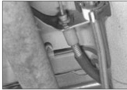
19.3 Handbrake rear cable fixed body location
