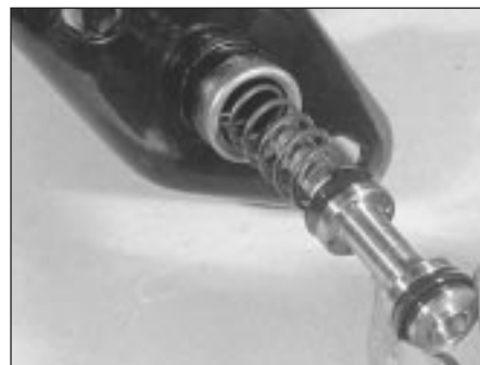
9.8b . . . followed by the secondary piston assembly
