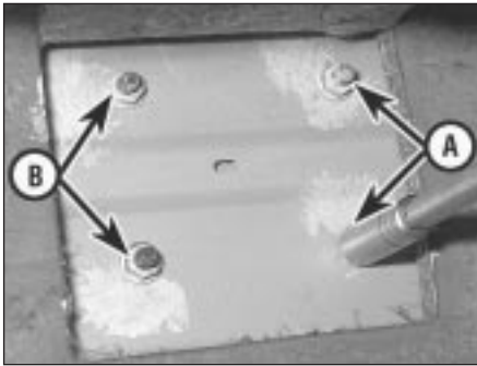
11.6 Servo mounting bracket retaining nuts
