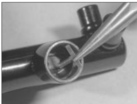
9.7 Removing the secondary piston retaining pin
