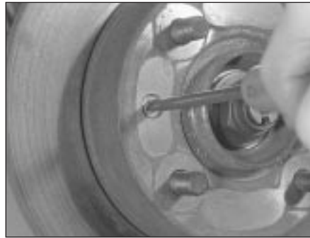
4.8a Extract the brake disc securing screw . . .
