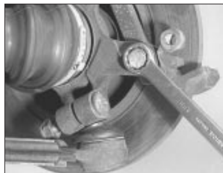
3.6 Undoing a brake caliper anchor bracket bolt
