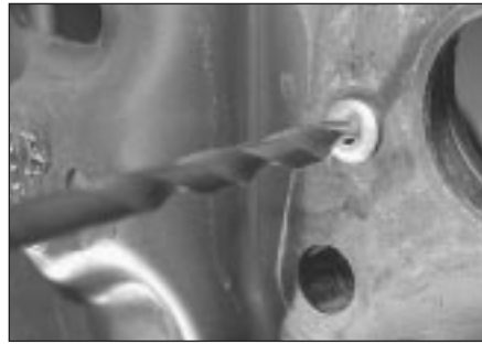
8.6 Drilling out a pop-rievt securing the brake backplate to the axle flange
