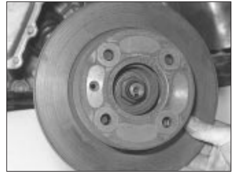
4.8b . . . and remove the disc from the hub
