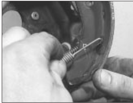
6.4a Detach the lower pull-off spring
